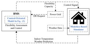
Fig. 2. Simulation Diagram.
