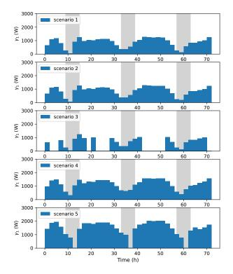
Fig. 4. Capacity of flexibility  $\gamma_1$  computed via (13) for different scenarios.
